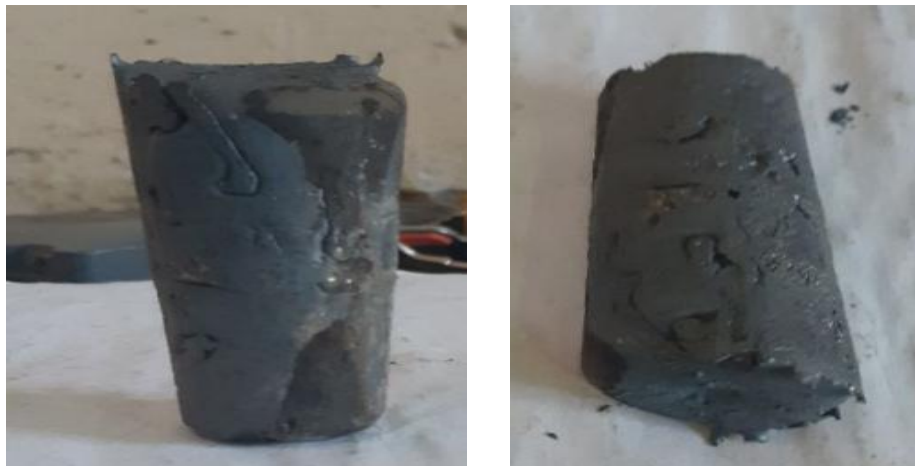
Figure 2. Samples cast in an electric arc furnace from a gray cast iron alloy in a sand-clay mold for research.
