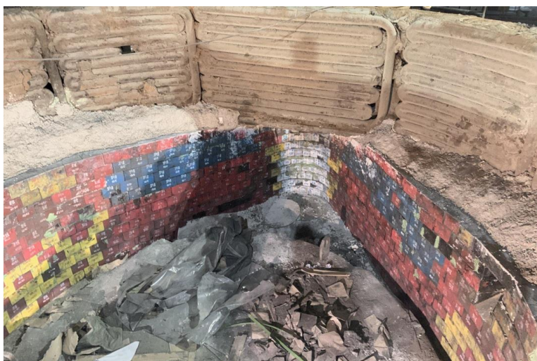
2 – picture. Electric arc furnace lining process
