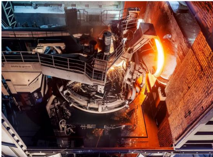
2 – picture. Electric arc furnace working process
