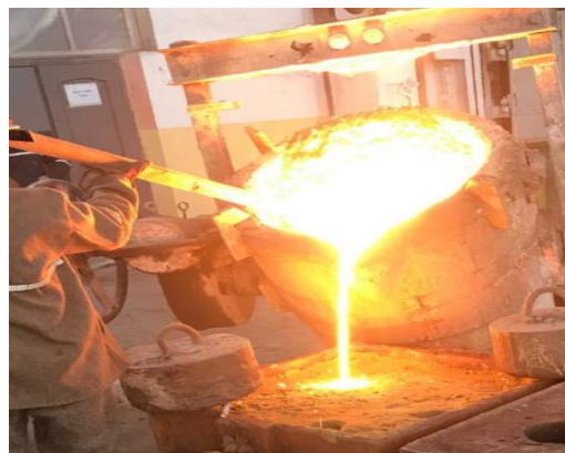
Picture 2. The process of casting a molded thin-walled lifting roof detail using a liquid glass mixture.
