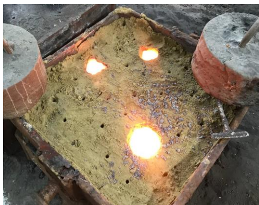
Picture 2. The process of casting a molded thin-walled lifting roof detail using a liquid glass mixture.
