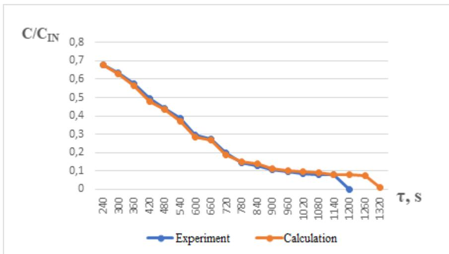
Fig.10. Comparison of experimental and calculated values of regeneration curves  $\text{Ca}^{2+}\text{-Na}^{+}$
