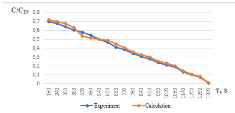
Fig.11. Comparison of experimental and calculated values of regeneration curves  $\text{Mg}^{2+}\text{-Na}^{+}$
