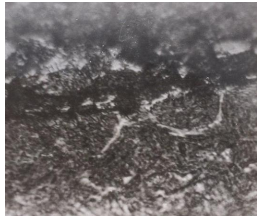
Figure 4 ε – phase along grain boundaries in the cyanidated layer x500
