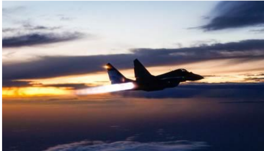
Pic.5 MiG-29B inflight with its Klimov RD-33 turbofan engines on full afterburner
