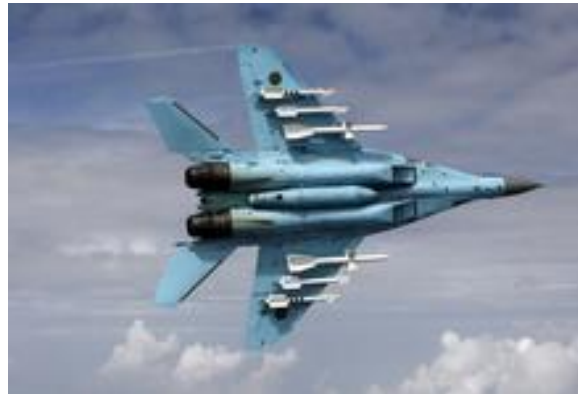
Pic.9 MiG-29B showing its full underbelly. Note the six underwing pylons carrying R-27 and R-73 air-to-air missiles. The centerline fuel tank is seen with an APU exhaust duct.
