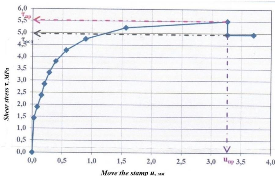
Figure 2. Dependence of Horizontal Displacements  $u$  of Stamp BS-7 on Applied Shear Stresses  $\tau$  at  $\sigma = 3.0$  MPa
