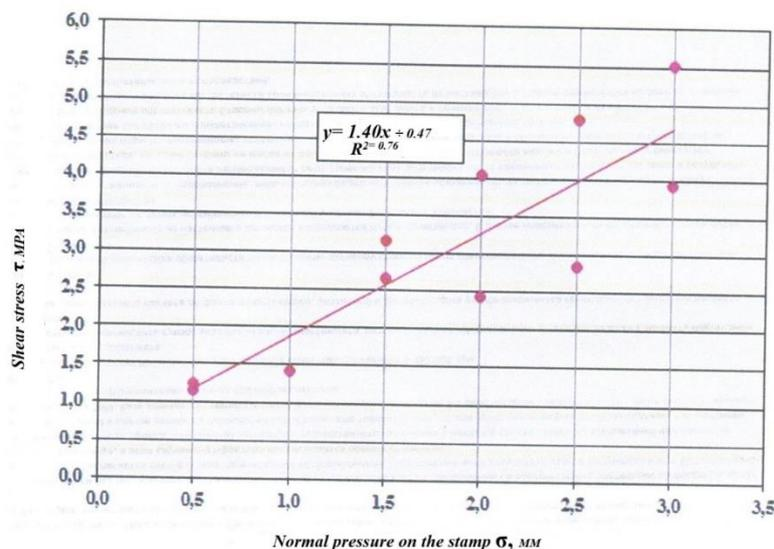
Figure 4. Dependence of Ultimate Shear Strength on the Magnitude of Specific Normal Load on Concrete Stamps BS-7 to BS-12
