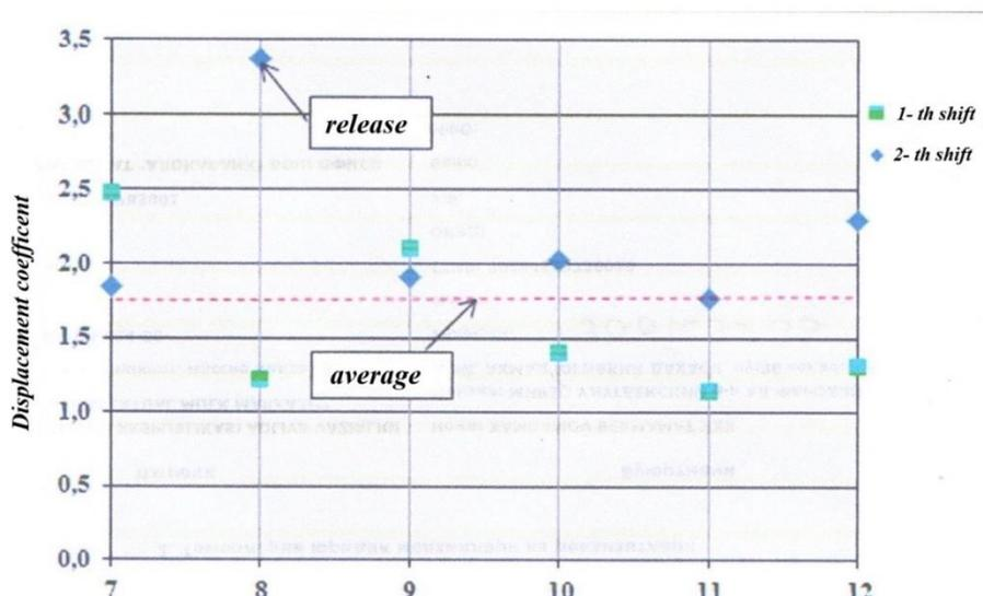
Figure 3. Shear Coefficients Obtained from Tests on Stamps BS-7 to BS-12
