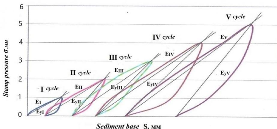
Figure 1. Example of Graphs  $s=f(\sigma)$  from Stamp Load Tests
