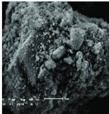
**Figure 4.2** SEM images of Strontium Nitrate Nanoparticles.
