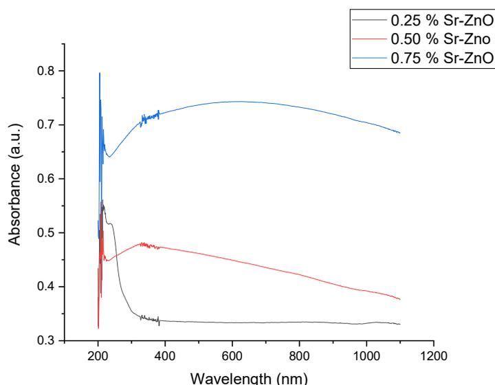
**Figure 4.10** UV-VIS Spectra of Doped ZnO Nanoparticles
