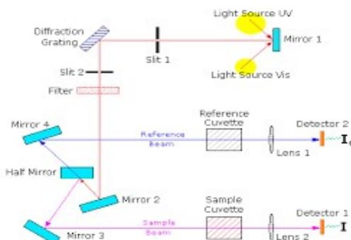
**Figure: 3.14** Diagram of a Spectrophotometer
