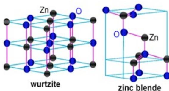
**Figure 1.2** Wurtzite ZnO Internal structure
