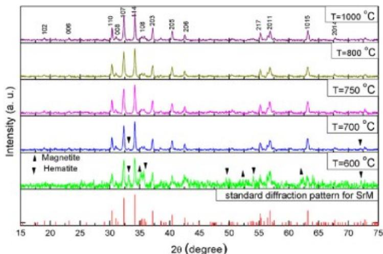
Figure 4.5 XRD Analyses of Sr Nanoparticles
