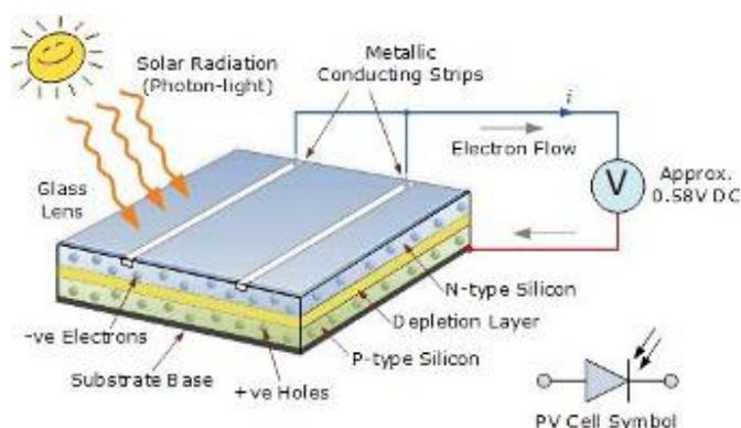
**Figure 1.3** Inside Photovoltaic cell working
