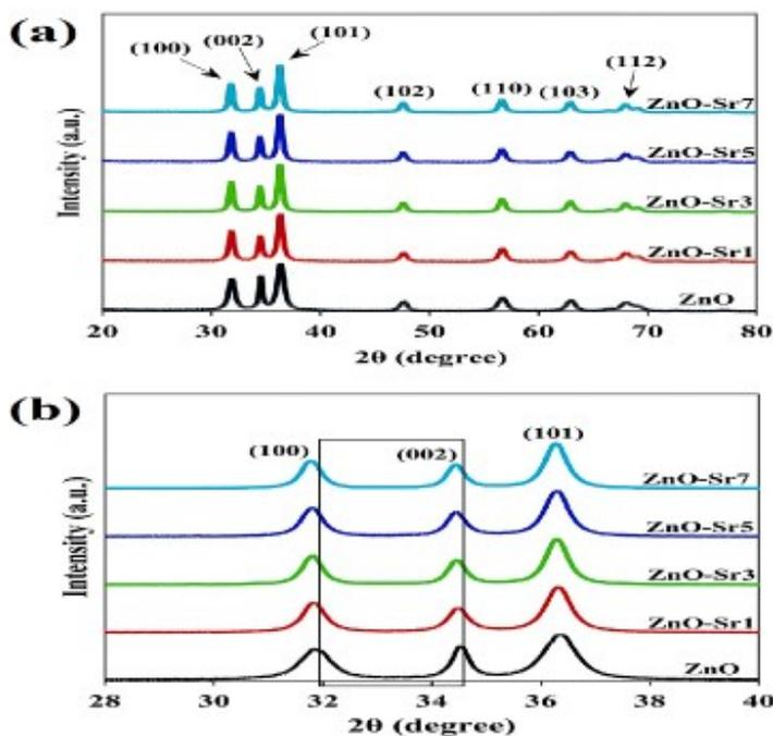
Figure 4.6 XRD Analyses of Sr doped ZnO Nanoparticles
