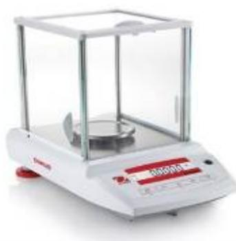
**Figure 3.2** Electronic Balance
