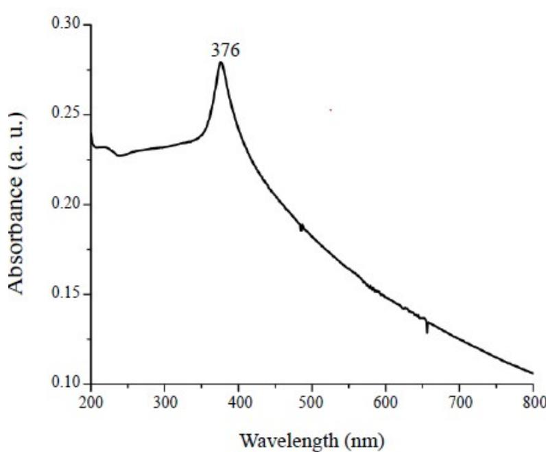
Figure 4.9 UV-VIS spectra of ZnO nanoparticles
