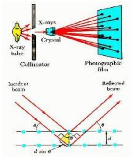
**Fig.3.12.** X-ray Diffraction Technique
