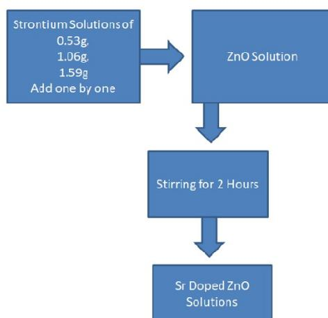
**Figure: 3.11** Synthesis process of Sr doped ZnO
