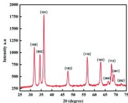
Figure 4.4 XRD Analyses of Pure ZnO Nanoparticles
