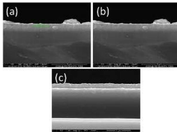
**Figure 4.3** SEM images of Strontium Doped ZnO Nanoparticles.
